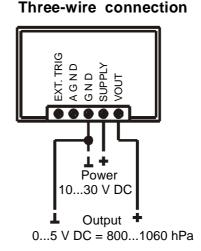
Both grounds (AGND and GND are in the same electrical potential in the barometer. Both three-wire and four-wire connections can be used; the four-wire connection must be used when the voltage drop in the supply ground line affects the pressure measurement accuracy. In normal operating mode no connection to the EXT.TRIG terminal is recommended. The barometers are protected against reverse operating voltage.
